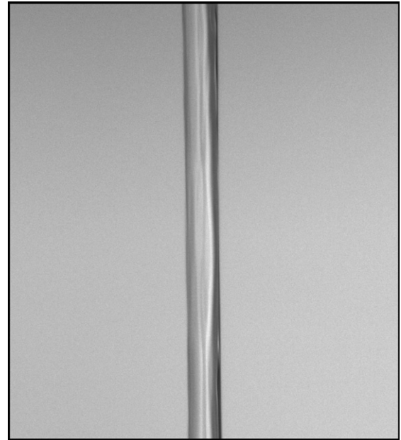
Fig. 2. A round nonturbulent liquid jet in still air (water jet, d_j = 1 mm, We_G = 0 , Re_L = 30,000 , and q = \infty ).
